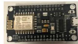
Gambar 3 Board NodeMCU ESP8266
