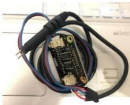
Gambar 1 Sensor *Total Dissolved Solids*
