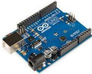
Gambar 1 Board Arduino
